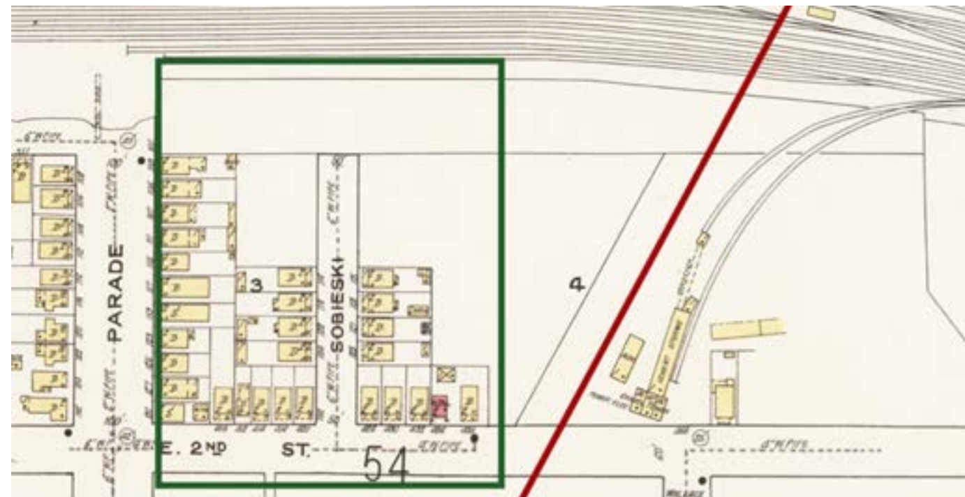
This 1921 Sanborn Fire Map shows that Standard Brick Works is no longer standing. Because of the construction of the “Mill Creek Tube,” a railroad spur was built to service the gravel and cement plant owned by Erie Concrete and Steel. The plant supplied the materials used to build the underground viaduct. The red line is the approximate location of the “tube.” The green square is the probable location of the French (1753) and British (1760) forts. (Library of Congress)
