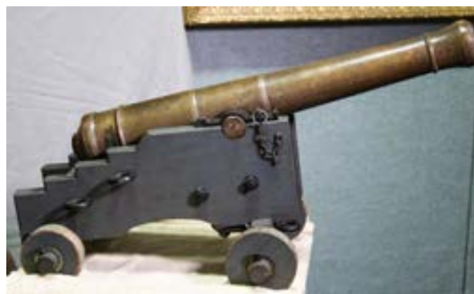
756 bronze French swivel gun reconfigured to mount on a naval gun carriage
