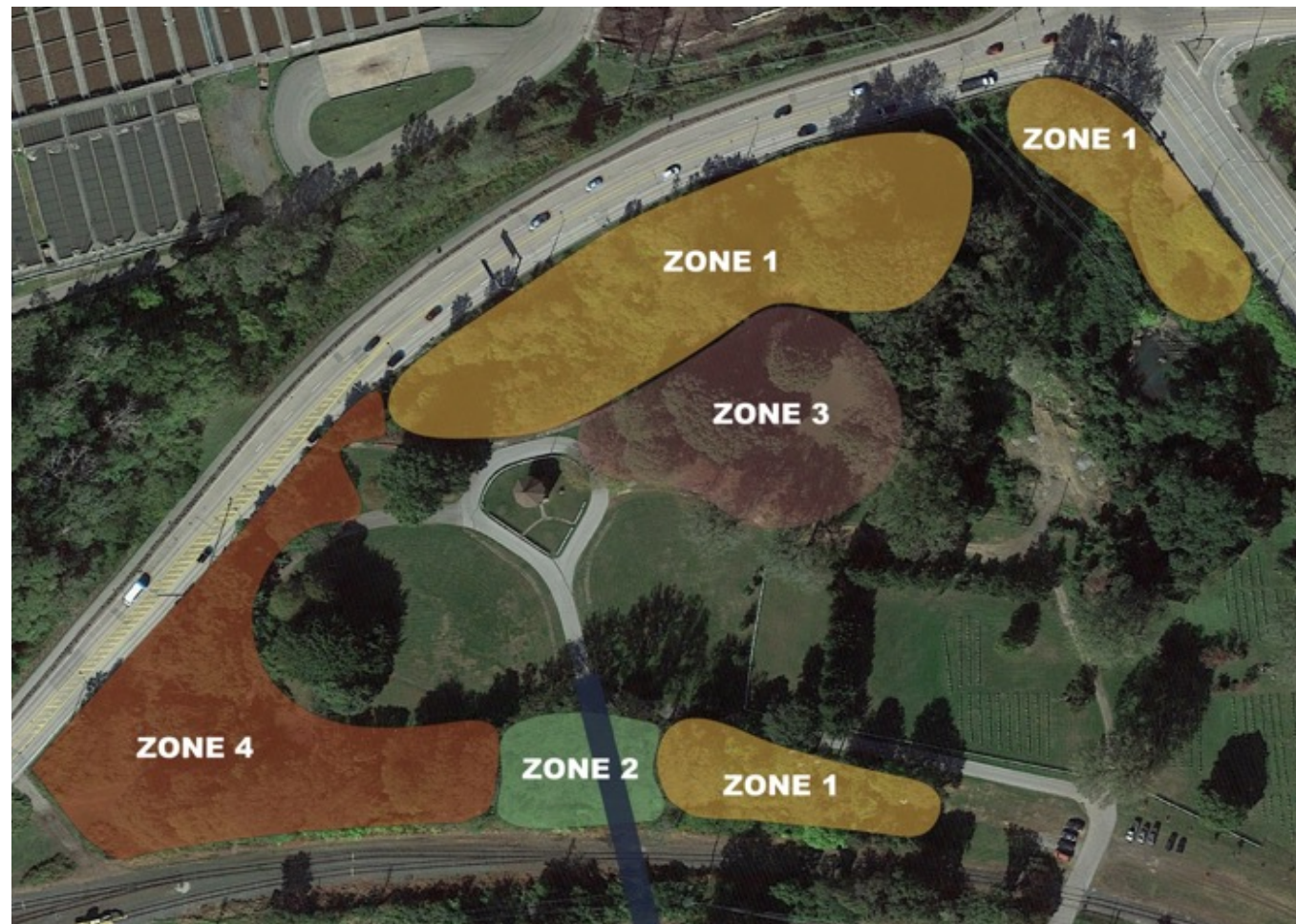
Any areas outside the identified zones should be maintained as a low tuft grass for ease of access to interpretive elements by all visitors, including handicapped. Care should be taken in removing trees. Root excavation can potentially damage archaeological resources.
